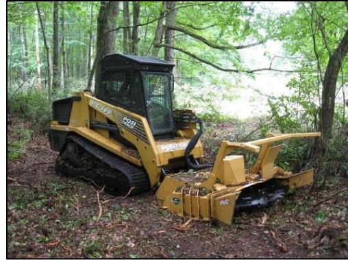
Figure 34. Skid Steer used to remove vegetation for mulching. Credit: ANF.
