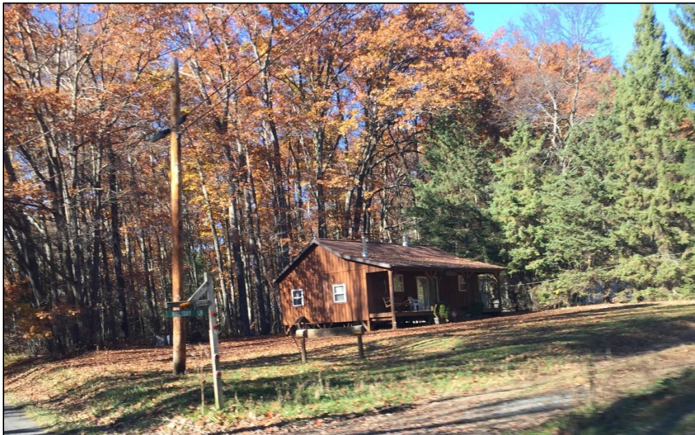
Figure 44. Trees overhanging a wood cabin, with heavy conifer component that could transmit fire easily from the ground to the canopy
