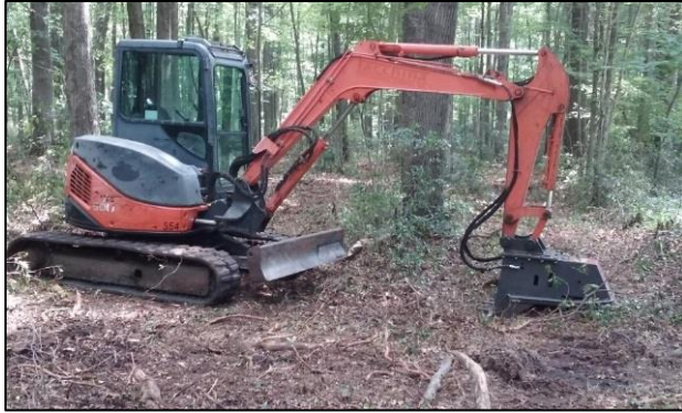
Figure 33. Hitachi mulcher used to breakdown piece size of cut vegetation. Credit: ANF.
